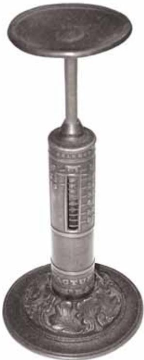
Figure 26a. ▲▲ This Ratcliff candlestick was seen in France. It was graduated in grammes and exported. The base is iron.
