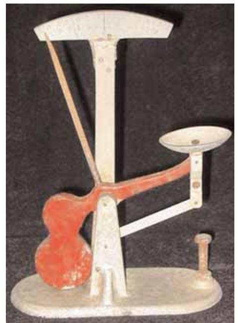
Figure 9. ^^ Zenith Prototype. Note the rounded ends and the lack of legs or leveling bolt.
