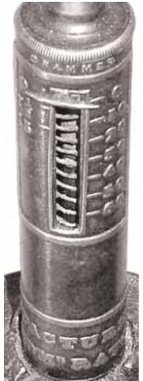
Figure 26b. ▲▲ Close-up of Figure 26a, showing the grammes from 0, 10, 20, 30, 40, 50, 60. The two positions for 7½ and 15 grammes (on the left side of the graduated plate) prove that it was intended for use in France.
