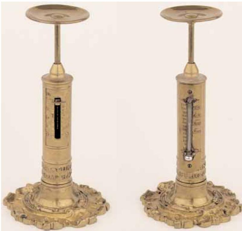
Figure 27. ▲▲ J & E Ratcliff candlestick with a thermometer screwed to the rear. The thermometer is much older than the 'stick, and has screws attaching it that are not the normal Ratcliff screws, so this is probably an extra added at some time during the life of the 'stick. As the thermometer plate is too long, it overlaps the stamped collar with their name on it, giving the piece an amateur look. Two 'sticks are known with thermometers on them. Postal rates 1840-65.
