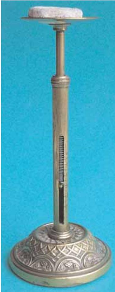
Figure 6. << Anonymous candlestick of exceptionally thin proportions, being 7½ inches (190mm) tall. The base is heavy, being an iron casting covered by a thin pressed brass ‘cup’.
