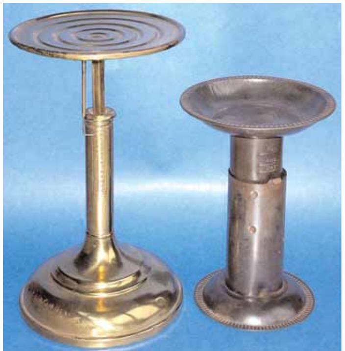
Figure 8. >> Two candlesticks for household use. The left-hand scale is an American scale by L E Brown of Cincinnati, patented in 1878. The long pointer can be adjusted in its length so that the scale is tared for a bowl.
