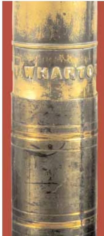
Figure 32. >> The tube of the candlestick shown on the Cover. The two grooves that are thought to characterise Wharton's work show distinctly. The seam is visible on the right side of the lower tube. The patina has worn away, showing that the black patina is not bronze but is a surface finish on brass.
