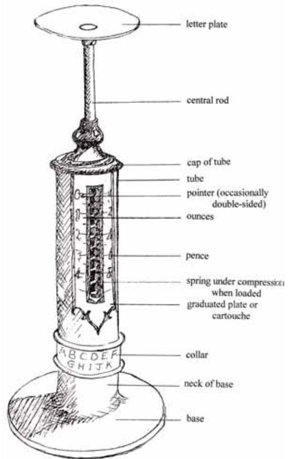
Figure 4. >> Diagram of the standard candlestick scale. The comment about the base refers to a sheet attached underneath, obscuring the view of the screw and the rod that descends as the load is applied. The spring under compression was the British method of utilising the spring. The spring under tension was more commonly used in the USA. The length of tube needed was not affected by this variation.
