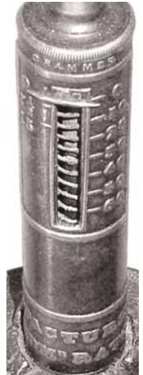
Figure 26b. ▲▲ Close-up of Figure 26a, showing the grammes from 0, 10, 20, 30, 40, 50, 60. The two positions for 7½ and 15 grammes (on the left side of the graduated plate) prove that it was intended for use in France.
