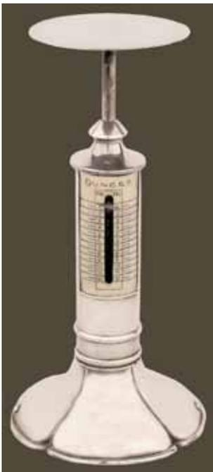
Figure 23. << Levi & Salaman solid silver candlestick hall-marked L & S 1904. They took out a design registration N°. 308820 for this elegant shape in 1897. The graduated plate is made of artificial ivory (celluloid), a material that is very prone to being wiped clean by the concientious housewife, leaving a blank sheet! Weight only, 0-12 oz.
